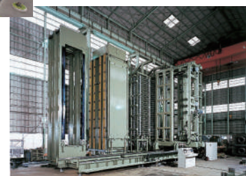
Top global share of multi-stage vacuum press machines for manufacturing copper-clad laminate (PCB material)
