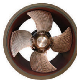
Side thruster used when a ship is departing or docking
