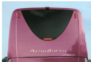
Polycarbonate resin window in the rear of a bus
