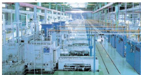
Fully-automated FA line that allows mass-production for the carburizing and quenching of a variety products
