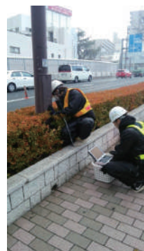
Taking measurements with only an ultrasonic sensor
