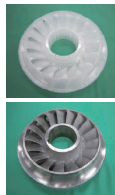
Stereolithography model from a 3D printer, and precision casting part from the model
