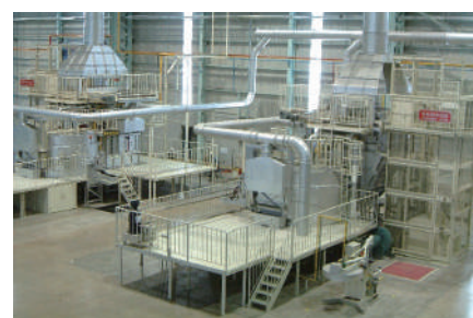
3 t/h tower aluminum melting furnace
