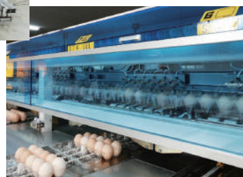
"SKY Series" egg washing, grading, and packaging system
