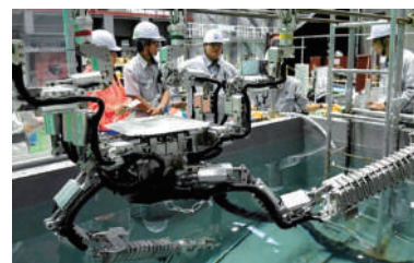
Robots for dismantling furnaces
