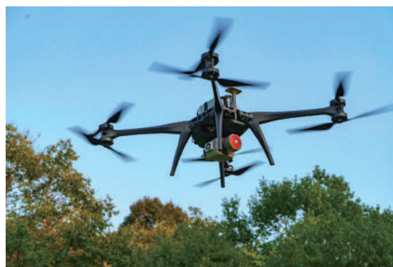
SPIDER-LX8 drone equipped with a 3D laser scanner
