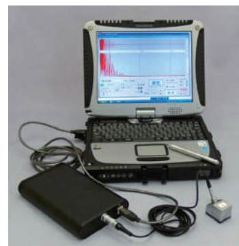
"NST-2" embedment depth measuring device
