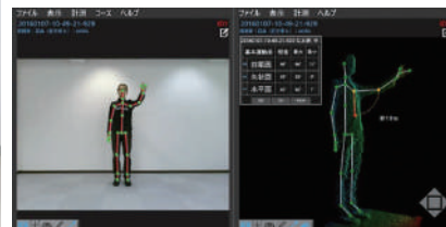
"Akira" Mobile Motion Visualizer for measuring the range of motion in joints (left) and 3D measurements using the device (below)
