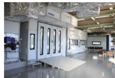
CAB-SP air-conditioned painting booth for car repair
